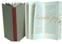
museum board, using an etching press. The 20pt board allows the paper to retain the debossment after it is glued down to the cover of the book. The binding used on this book is a sewn board structure originally devised by Gary Frost. grey stamped paper over boards, red cloth spine and tips, title
