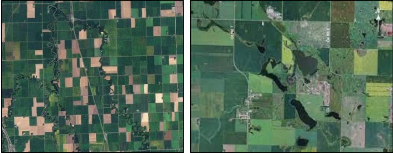
Figure 4: Aerial photographs of the rectangular survey system in Ohio (left) and North Dakota (right)
