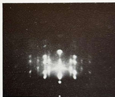
Figure 5. Specimen as for Figure 3 after a total exposure of fifteen minutes to the electron beam. Mica [100] azimuth
