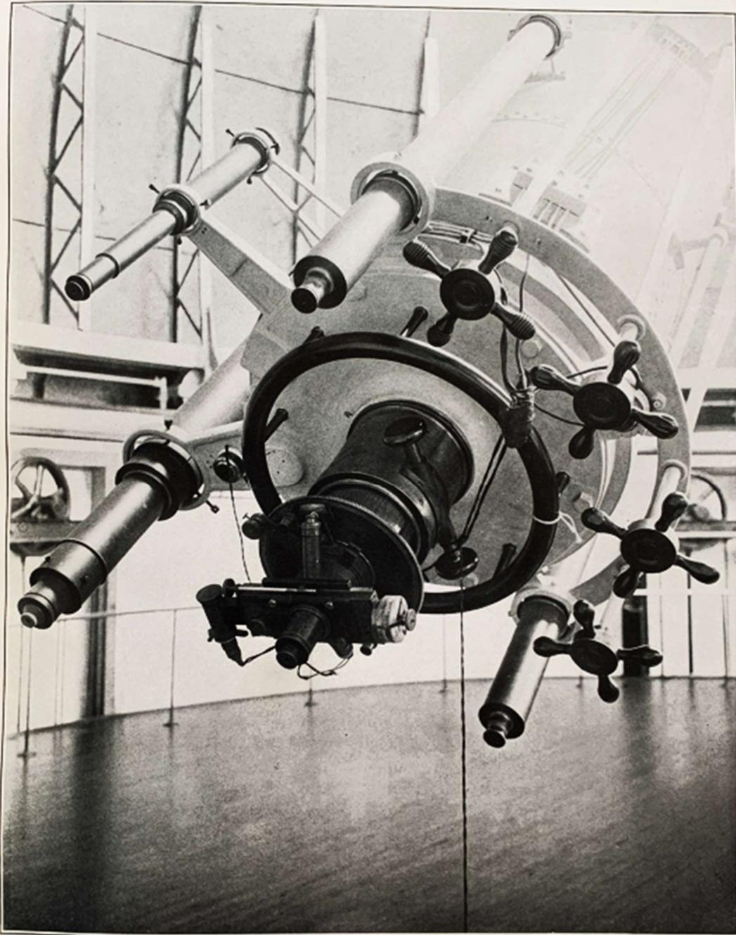
THE EYE-END OF THE 26-INCH EQUATORIAL—SHOWING THE MICROMETER, TWO FINDERS, TWO MICROSCOPES FOR READING THE DECLINATION CIRCLE, CLAMP AND SLOW-MOTION HANDLES, AND FOCUSING RACK.
