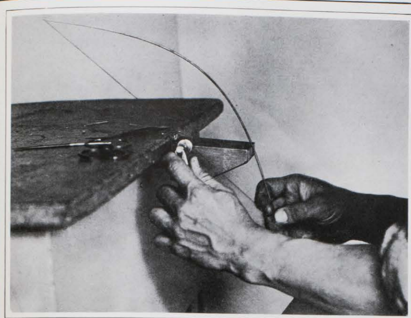
Drilling a pearl by means of the bow-drill
